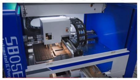
Robotic IC programming reduces cost and turn-around time for custom-programmed microprocessors and memory chips used in printed circuit board assemblies made in the USA.
