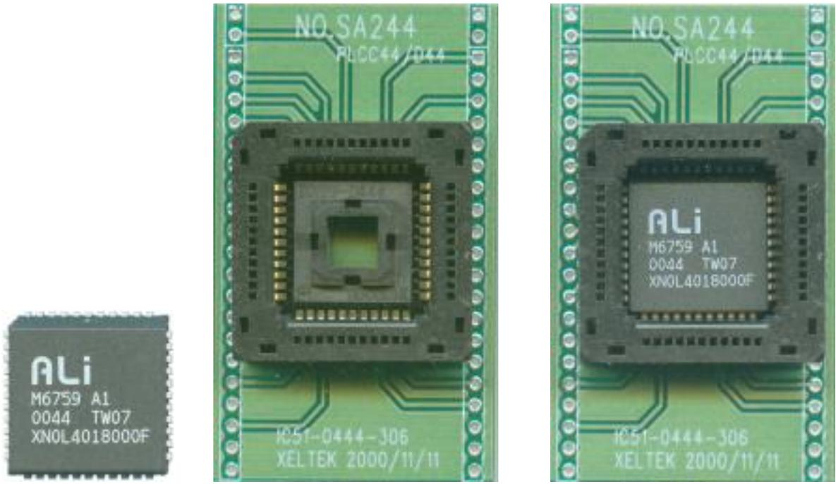
·Adapters are inserted in the same way as DIP devices.
