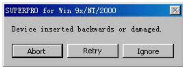
Please take out the chip and insert again properly. If the problem still exists, the chip may be damaged or non-functional.
