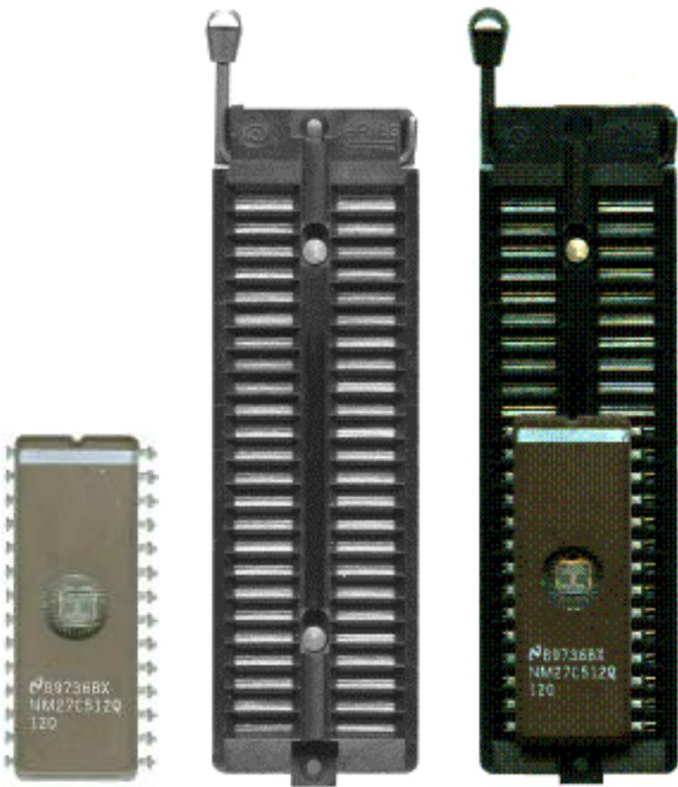
·None-DIP: Socket adapters are available for PLCC, QFP, SOIC etc. Insert the chip according to the instructions in the Adapter Information box. The insertion follows the position of pin 1. It is necessary to identify the pin 1 of the chip. In the Adapter Insertion dialogue box, there is a solid square, which indicates the position of pin 1.
