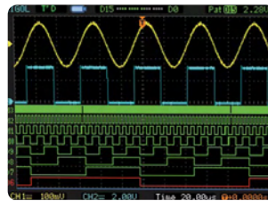
Pattern Trigger The trigger condition is a combination of the level of the signal and the edge
