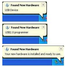
4. After you open the application software for the programmer, the system automatically starts the initialization. If it does not, make sure the programmer is securely connected to the computer and that the power switch is on.
