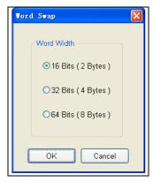
Select the **Word Width** option to swap high byte and low byte according to the specified width in the address range and select **OK**. Otherwise, select **Cancel**.
