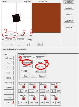
Select the Socket Adapter where the chip is inserted under Device (#1). Now click M.Camera(#2) for the Nozzle to pick up the chip and bring it over to the upward camera.
