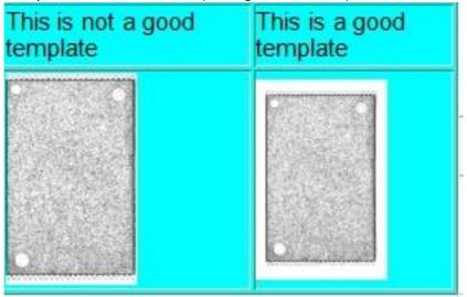
**2)**The background must be completely white, or it will highly fail vision check. To adjust the background color, we want to adjust the camera's contrast. Adjusting the contrast can be done on the Upward camera.
